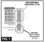
Тο program vour BirdXPeller PRO unit you will need a small screwdriver, toothpick, or other pointed, rigid object to move the switches in the switch arrav (see FIG. 1). The switch arrays are the switch banks
